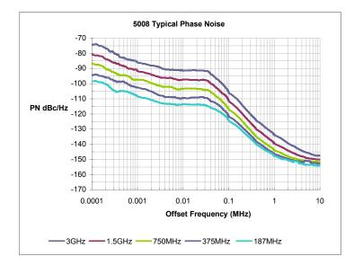
Phase noise was measured using the internal 10MHz reference with the Phase Detector Frequency set to 10MHz. The Frequency Increment was set to 1000kHz. The Charge Pump Current setting was 5mA.
